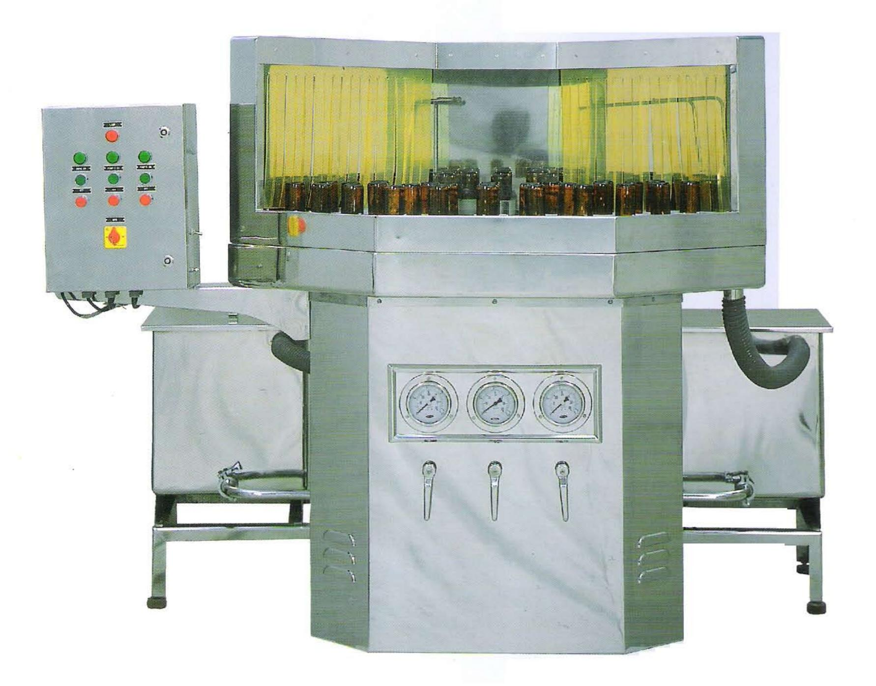
Rotary bottle washing machine give you perfectly clean the bottles washing to suit highest standards of the industries. The machine suitable for Pharmaceuticals, food, distilleries and allied industries.
